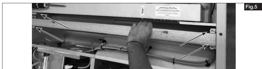
4. Remove support plate if necessary (see Fig. 5).
